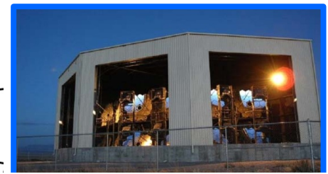
Segmented mirrors 256 hexagonal PMTs/camera
