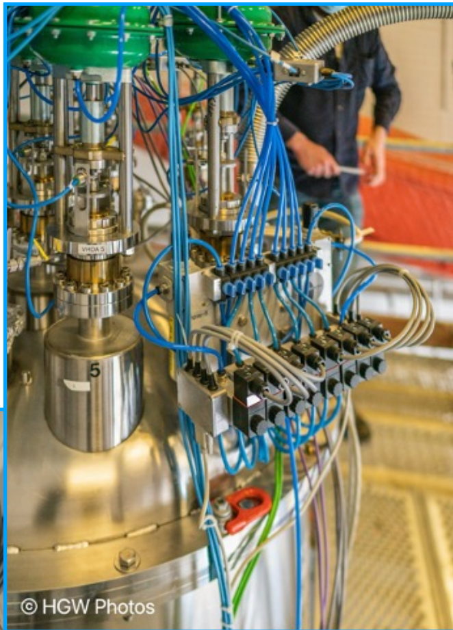
Fully instrumented condenser system
