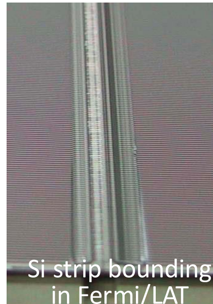
Detail of the detector-ASIC bonding in the AGILE Si Tracker
