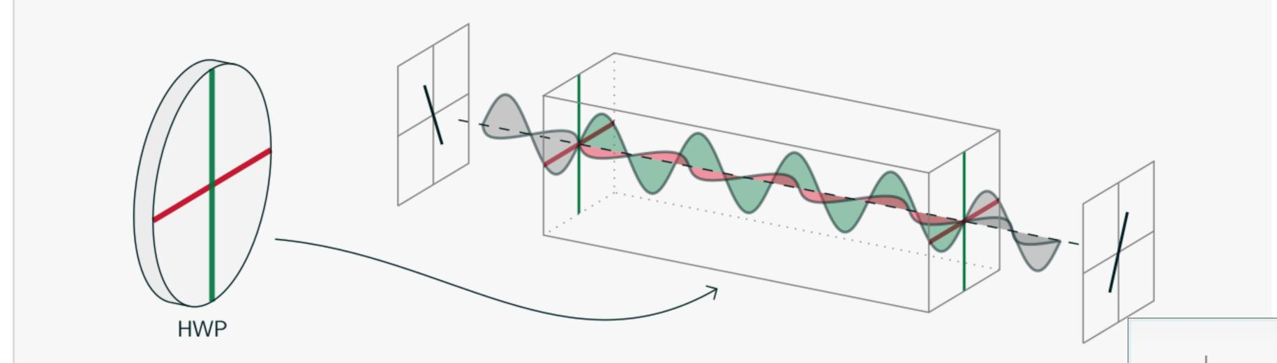
A rotating (ideal) HWP modulates the intrinsic polarized signal at  $4f_{\text{HWP}}$ , and can help to control systematic effects:
