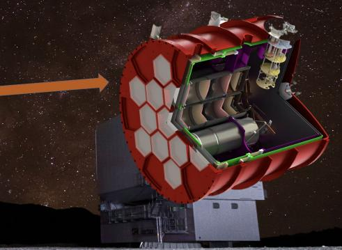
Large Aperture Telescope (LAT) 6m
