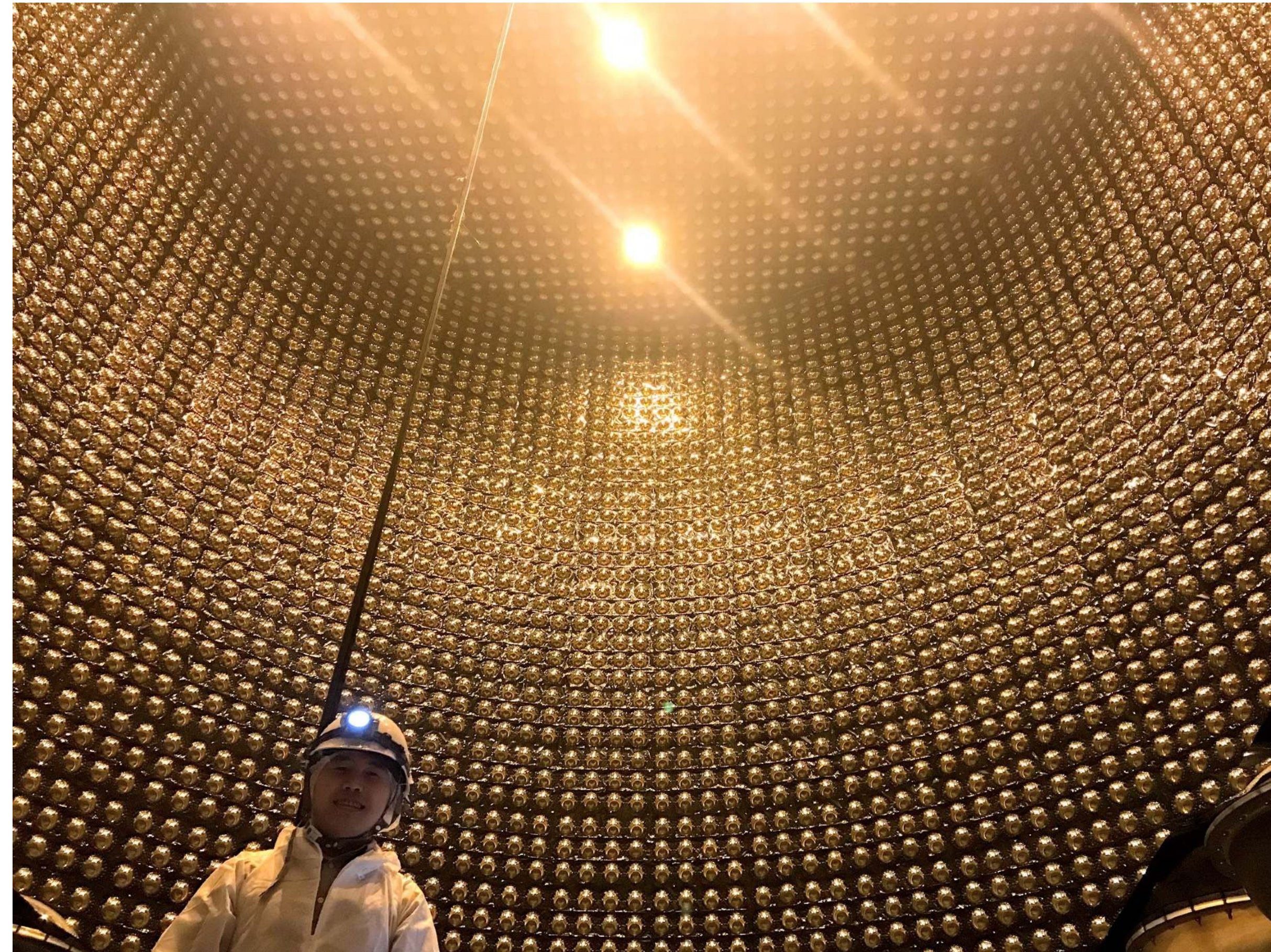
SC in Super-K for refurbished work in 2018 before doping Gd for new observation period
