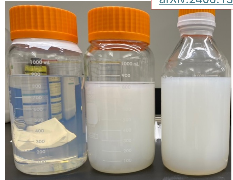
Three samples of opaque water-based liquid scintillator (oWbLS) with different scattering lengths
