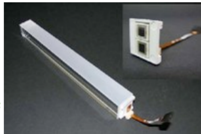
ES : silicon strip sensors strip width 1.9mm
