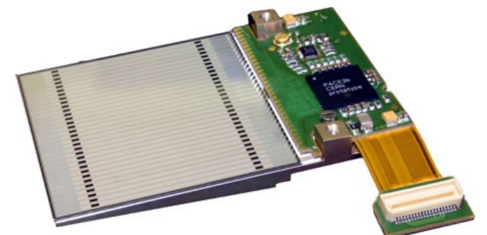
ES : silicon strip sensors strip width 1.9mm
