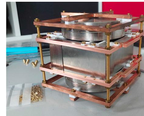
Cage structure mock-up ready for mechanical tests
