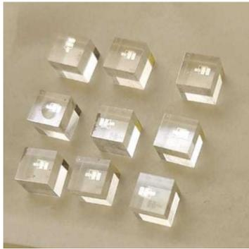
W-TES on  $\text{CaWO}_4$  detector with transition temperatures of 12-15 mK
