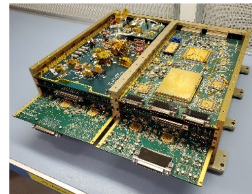
Instrument Electronics EM unit assembled FM boards mid-delivery
