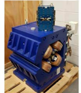
Permanent magnet quadrupole prototype (top) for SOLEIL II and Electromagnet quadrupole for SOLEIL
