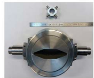
BPM prototypes for SOLEIL (bottom) and SOLEIL II (top)
