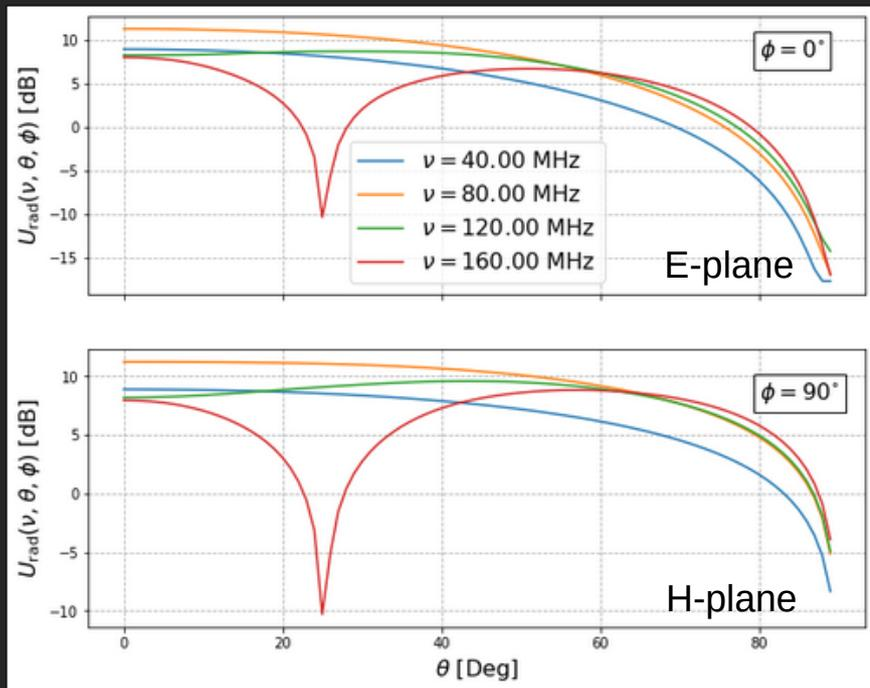
Typical broadband dipole antenna beam
