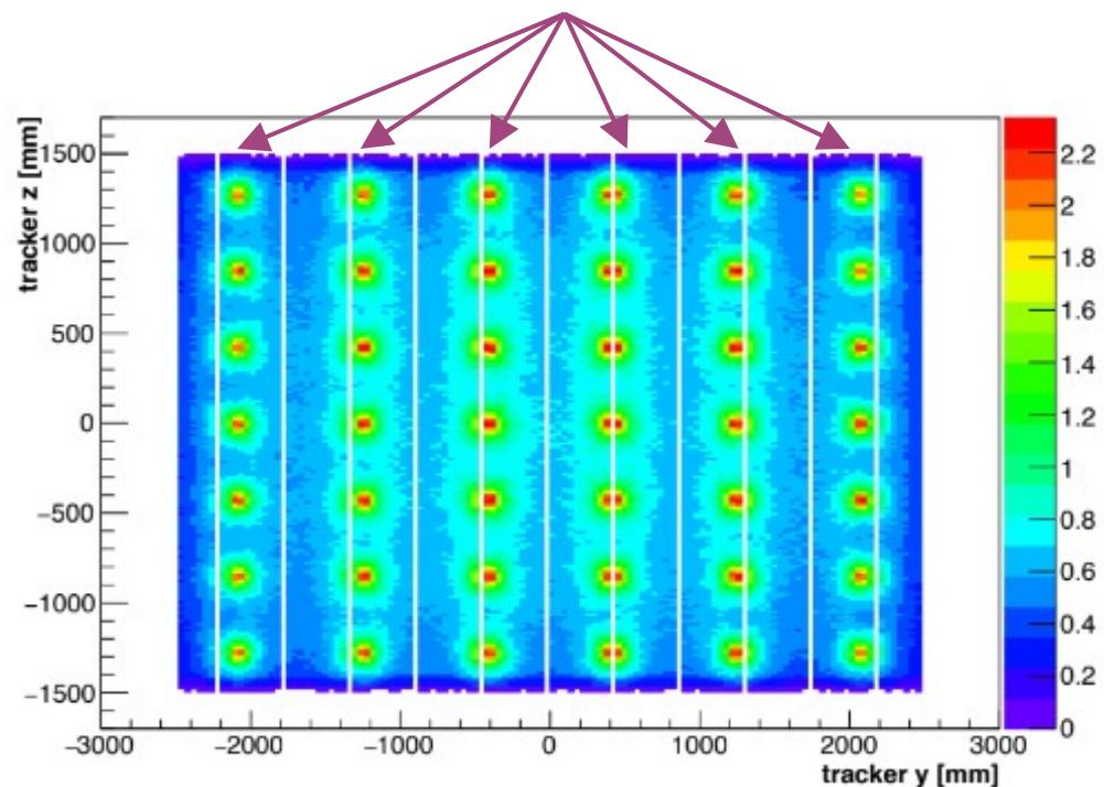
Perform calibration with the two internal conversion electrons of  $^{207}\text{Bi}$
