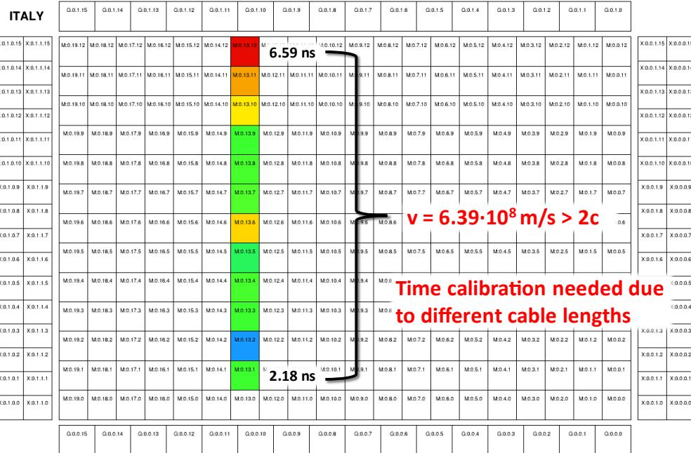
Time calibration needed due to different cable lengths
