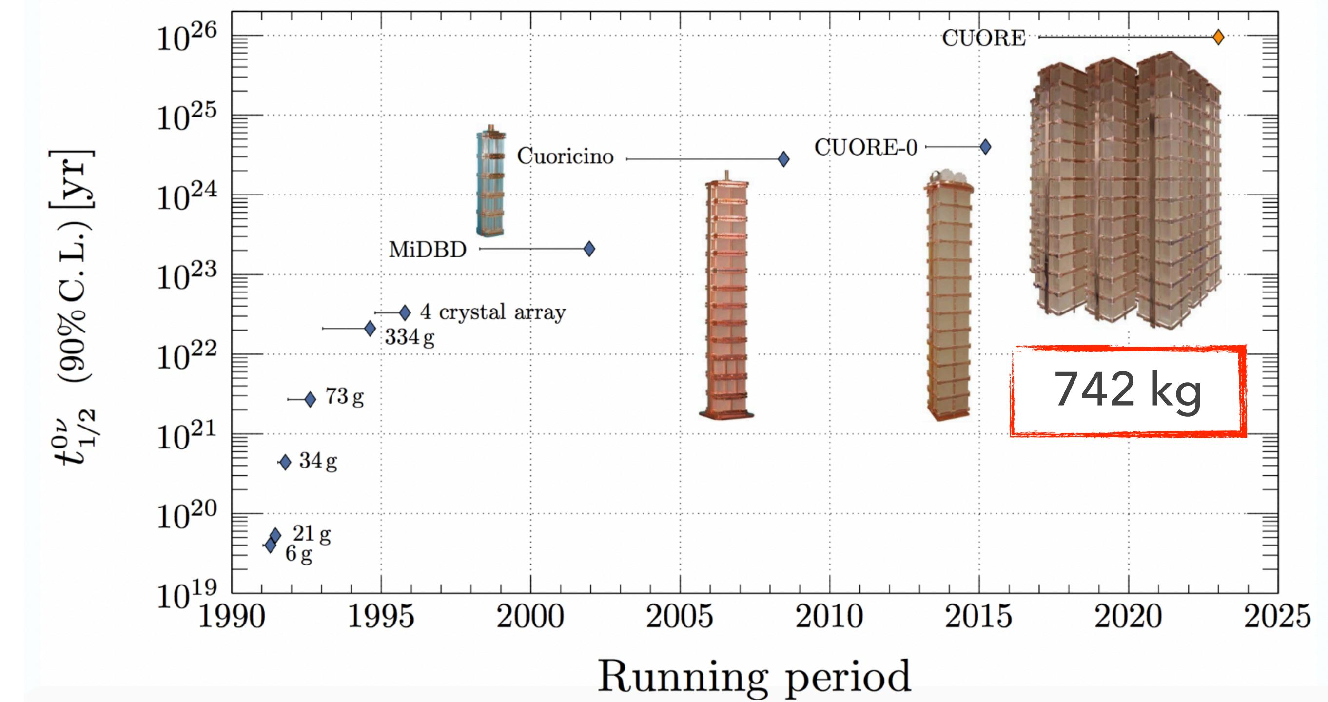
Starting from a few grams → 30 years of technical development for crystal growing, low temperature cryogenic, material handling, computing resources,...
