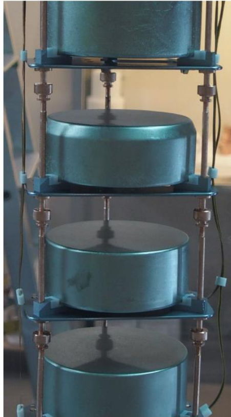
New low-mass detector holders (Si, Cu, PTFE)
