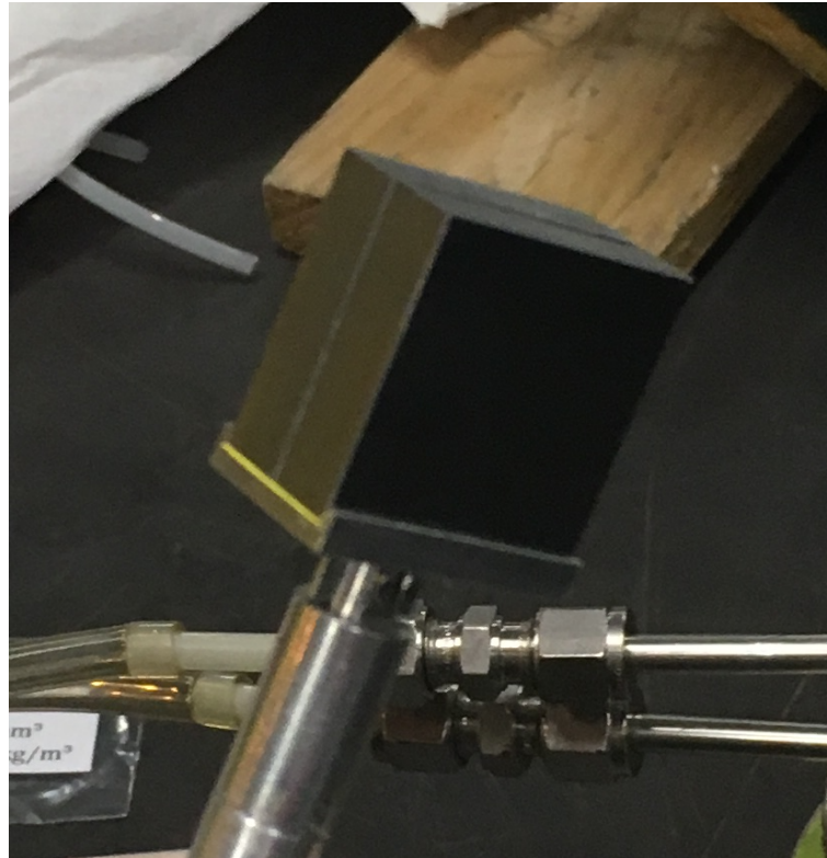
1.5 cm thin graphite target
