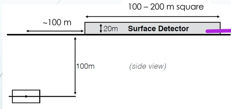
Proposed large area **surface** detector above an LHC pp IP dedicated to detection of ultra long-lived particles - air decay volume with **tracking chambers**
