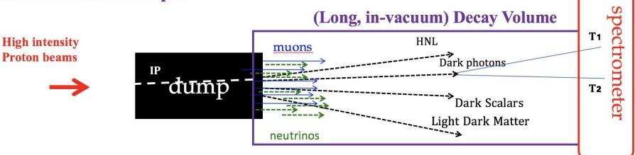
Crucial ingredients to disentangle signal from background: <u>timing</u> (T1-T2) and <u>pointing</u> (IP) (in addition to Veto and PID systems).
