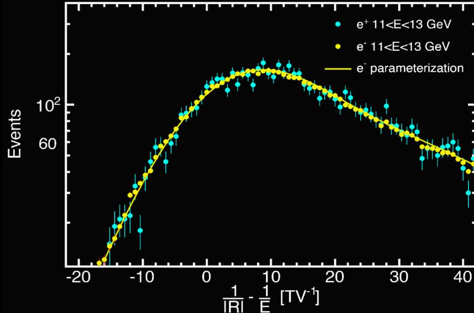
**The accuracy of the rigidity scale is found to be  $0.033 \text{ TV}^{-1}$ , limited mostly by available positron statistics.**
