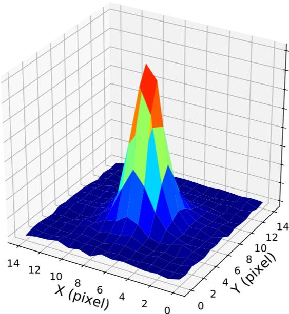
**PSF → light spreads due to optics and the atmosphere**
