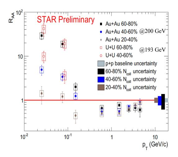
$R_{AA} \sim 30\text{-}40$ at  $p_T < 0.05$  GeV/c in 60-80% central Au+Au and U+U
