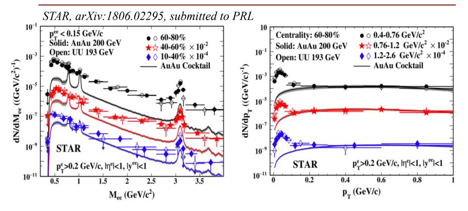
Significant enhancement of dilepton yield at  $p_T$ <0.15 GeV/c in (semi-)peripheral Au+Au and U+U collisions
