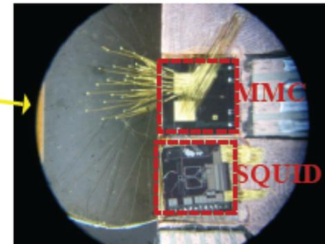
**Sensor technology** Metallic Magnetic Calorimeter
