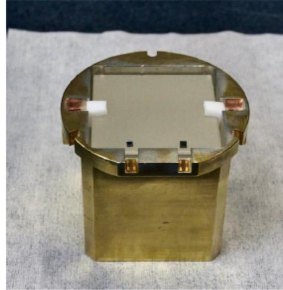
GeCo1 has also been tested coupled to a natural  $\text{TeO}_2$  crystal (784 g) at a working temperature of 17 mK
