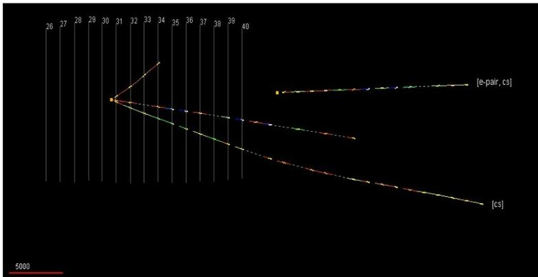
■ **Scan-back:** CS-tracks are followed upstream from film to film to find the n-interaction vertex
