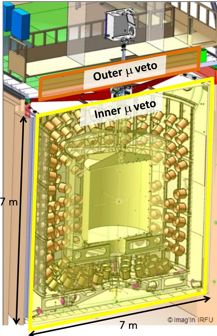
A concentric arrangement of cylindrical sub-detectors...
