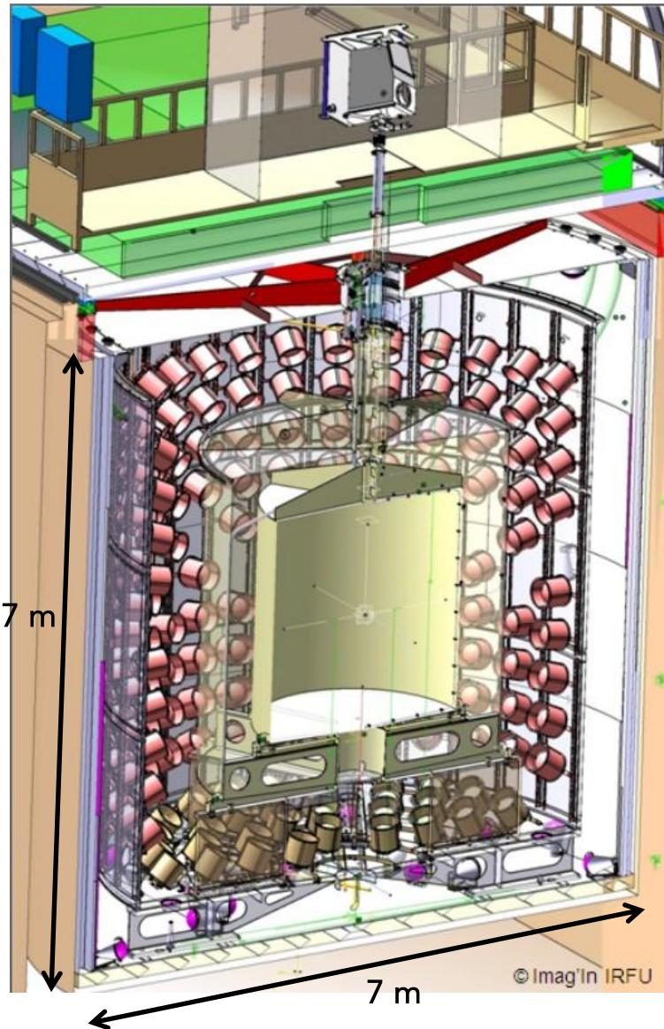
A concentric arrangement of cylindrical sub-detectors...
