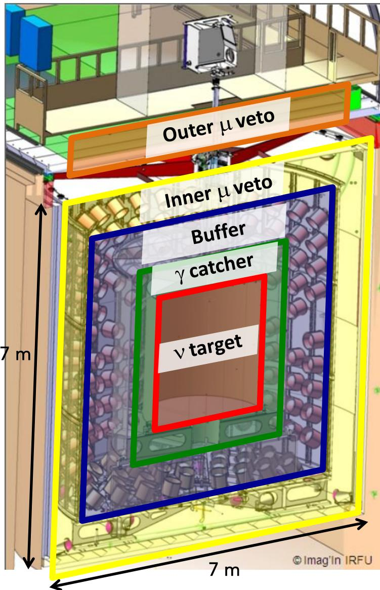
A concentric arrangement of cylindrical sub-detectors...
