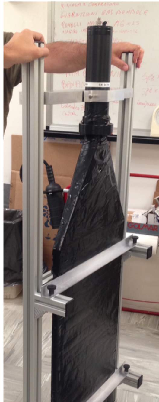
Outer Veto: plastic scint. + Light guide + PMT
