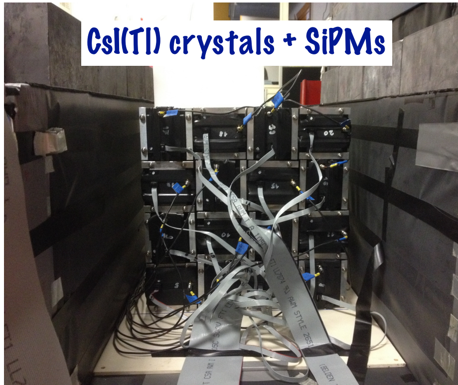
Inner Veto in the lead vault
