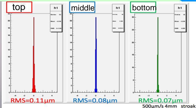
Repeatability for driving in each stage is well below 0.5μm.
