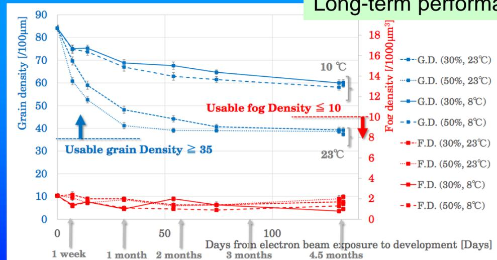
Initial and long-term performance of new emulsion gel is kept at safety level for signal and noise.
