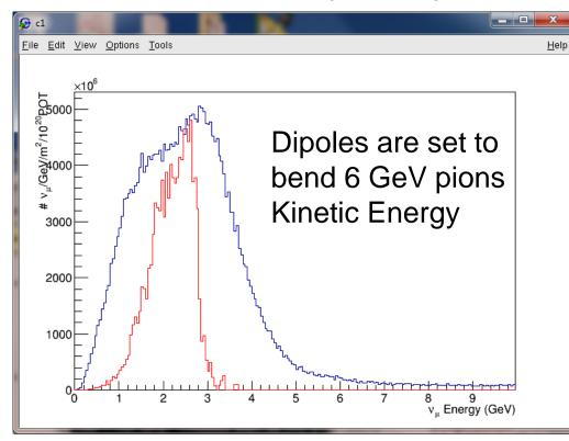
In presented concept, two bending magnets are identical, C-dipoles, conventional, iron dominated with field ~0.5T, ~2.4m long, gap 0.6 m and 1m field width. The first dipole is 0.2m separated from both horns. None of used parameters are optimized.
