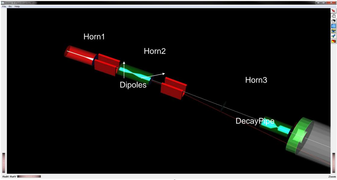
In any existing neutrino facility there is about 25 meters from start of Target to the entrance to Decay Pipe inside of Target Hall. The aim is to make minimal modification and utilized existing/planed facility
