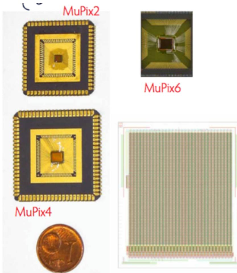
5 generations of prototypes, MuPix7 is current generation with all features of final sensors
