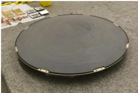
Thin, low loss, high thermal conductivity alumina filters and lenses with epoxy-based antireflection coating
