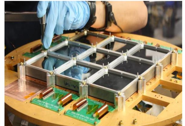
Plug & play detector modules each have 64 dual-pol 95 GHz camera pixels and contain cold multiplexing electronics.
