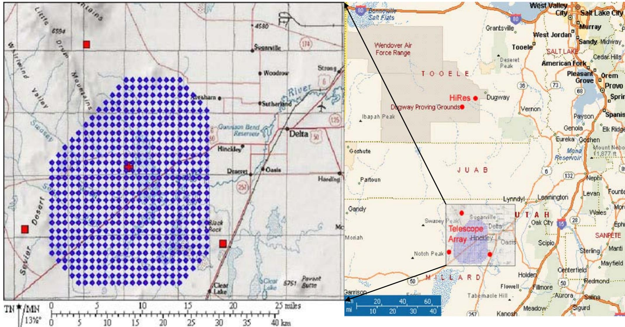
The High Energy component of Telescope Array – 38 fluorescence telescopes (9728 PMTs) at 3 telescope stations overlooking an array of 507 scintillator surface detectors (SD) - complete and operational as of ~1/2008.
