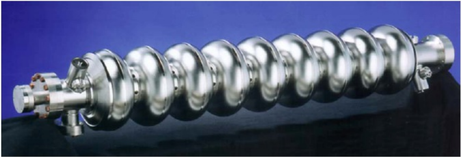
Figure 1.2-1: A TESLA nine-cell 1.3 GHz superconducting niobium cavity.
