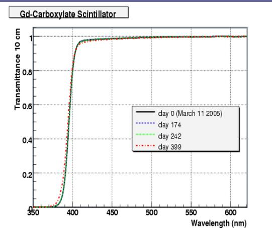
Test of the long-term stability of Gd-doped LS samples
