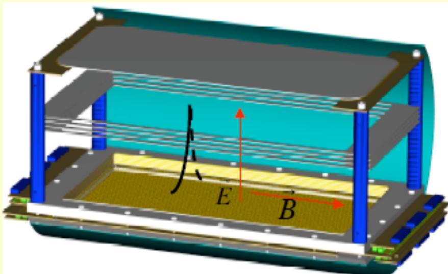
Width 300 mm, height 150 mm, drift length 150 mm
